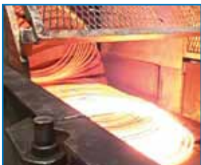
Loop cooling conveyor
