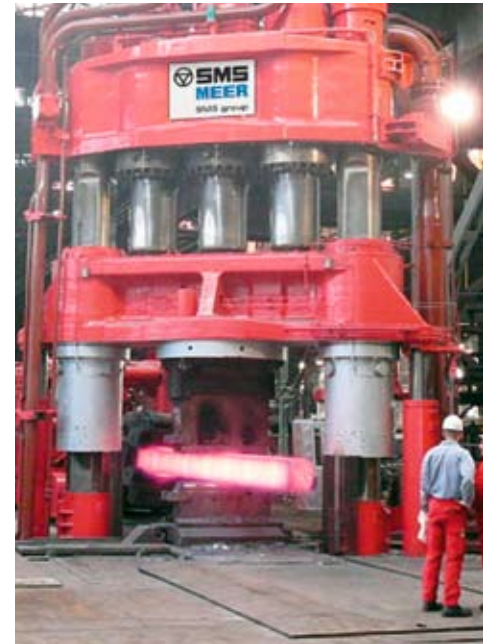
Open-die forging press after repair and modernisation
